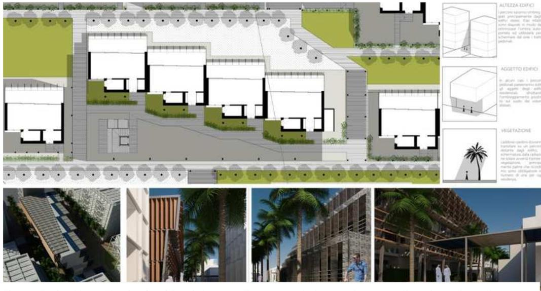
Fig. 6 - Project hypothesis of residential areas. The general plan and perspective views show the effect of the mutual sliding of the apartments to obtain sun protection and avoid introspection. This also allows, together with the vegetation, the shading of the pedestrian paths and common
