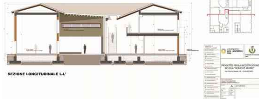
Fig. 8. Project of the new school “Romolo Murri” of Gualdo. Cross section of the open space-cloister in the middle and of the covered space-Agorà. The maximum height are 7.43 m at the eaves extraction and 9.16 m at the top higher (source: L. Notarantonio 22/09/2017).
