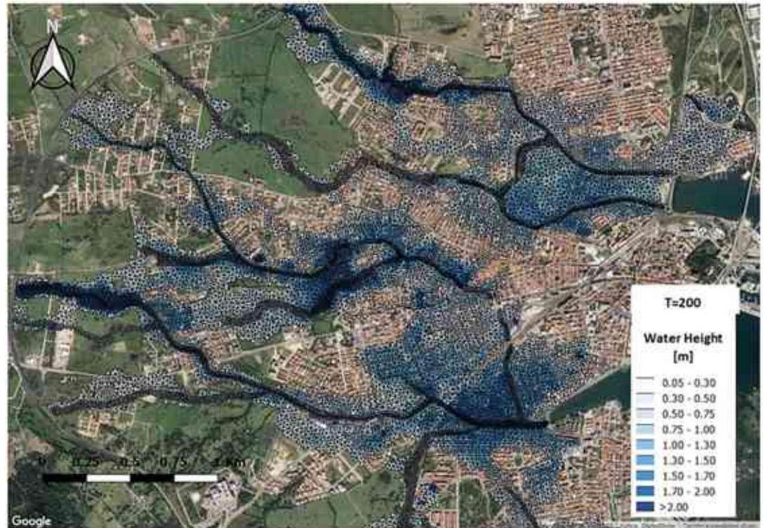
Fig. 3. Hazard layer: flood map related to a 200-year return period flooding scenario. The same maps have been developed for different year return period (50-100-500).
