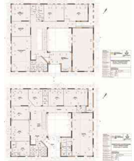
Fig. 6. Project of the new school "Romolo Murri" of Gualdo. Plan of the ground floor with the open space-cloister and a covered space-Agorà for socialization, 3 classrooms for primary school, a classroom for kindergarten school, a gym, a kitchen, a canteen, toilets. Plan of the first floor with 2 classrooms for middle schools, 2 laboratories, a multipurpose room, a teachers room, a library (source: L. Notarantonio 22/09/2017).
